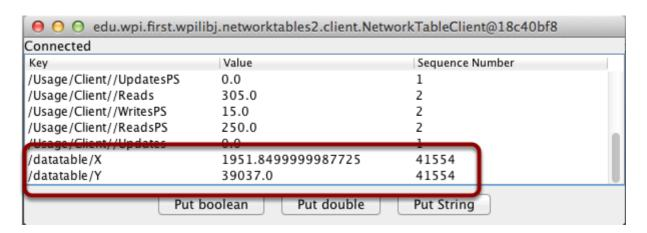
There is a diagnostic tool called TableViewer that will display the current state of the NetworkTables table. In this case, running it will show the current values of all the variables in the variables created in this example are shown in the red box above. TableViewer is located in the sunspotfrcsdk folder for NetBeans intstalls or in the C:\WindRiver\Workbench\WPILib folder for C++ installs.
