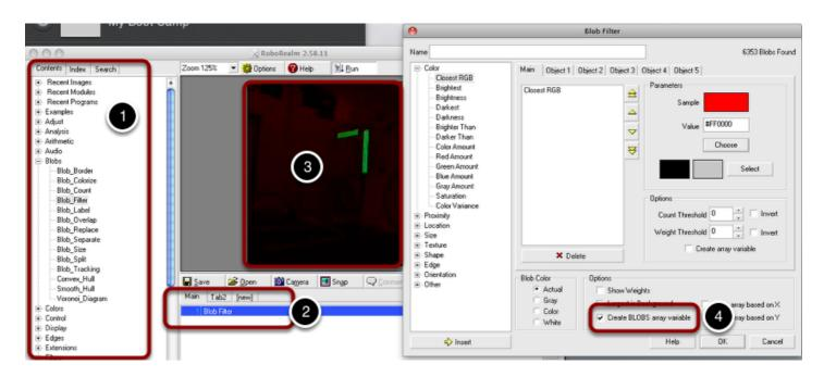
Create the RoboRealm program using the image processing elements shown in the "Contents" tab (1) on the left side of the interface. The program will appear in the bottom window (2). You can drag images from Windows Explorer into the Image window (3) to make sure that your algorithm works well and is repeatable for all the positions that the robot might be in.
