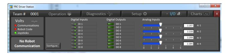
The same Driver Station methods can be used to interact with Virtual IO if no Cypress Board is present. On the IO tab of the Driver Station there are controls for each of the 8 Digital Inputs (click to toggle), indicators for the 8 Digital Outputs, and controls for the 4 Analog Inputs (click and drag or type in the box to set).
