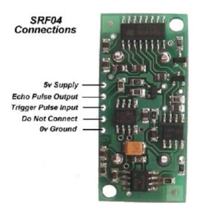
To aid in the sue of Ping-Response Ultrasonic sensors such as the Devantech SRF04 pictured above, WPILib contains an Ultrasonic class. This type of sensor has two transducers, a speaker that sends a burst of ultrasonic sound, and a microphone that listens for the sound to be reflected off of a nearby object. It requires two connections to the cRIO, one that initiates the ping and the other that
