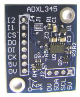
The ADXL345 is a three axis accelerometer provided as part of the sensor board in the 2012-2014 KOP. The ADXL345 is capable of measuring accelerations up to +/- 16g and communicates over I2C or SPI. Wiring instructions for either protocol can be found in the FRC component datasheet.
