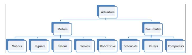
The chart shown above outlines the types of actuators which can be controlled through WPILib. The articles in this section will cover each of these types of actuators and the WPILib methods and classes that control them.
