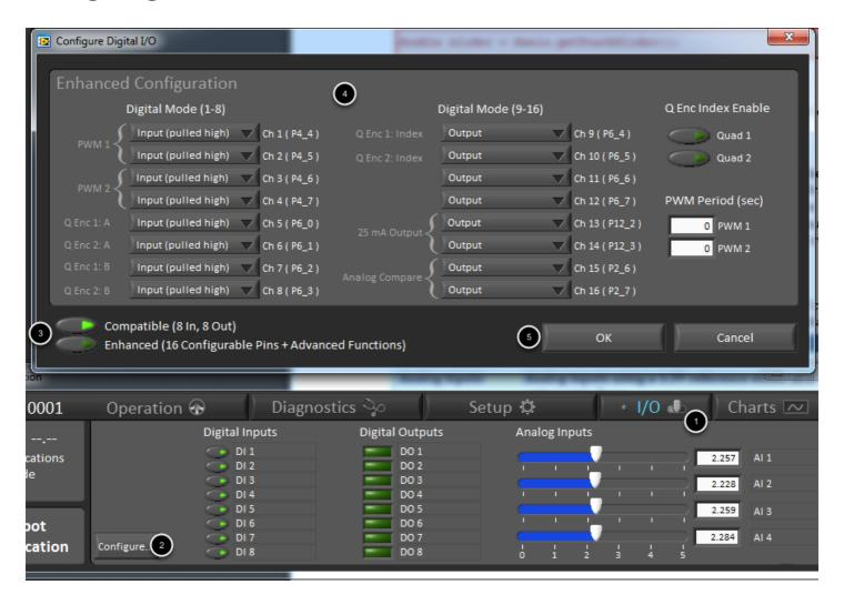
The Cypress board can be set to one of two modes when used with the FRC Driver Station. Additionally, the function of each pin and another of other advanced features can be configured if the board is set to advanced mode. To set the mode of the board, click on the I/O tab of the Driver Station, then click the Configure button. Select Compatible or Enhanced at the bottom of the dialog,
