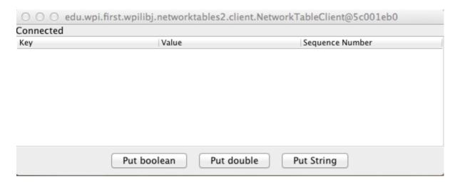
The TableViewer will start up and show all the keys (variable names) and values for those keys. In addition it shows a sequence number which is an internal NetworkTables field used to determine if values are updated and need refreshing. The sequence number increments every time the value of a NetworkTable variable changes. The values wrap around at 65535.
