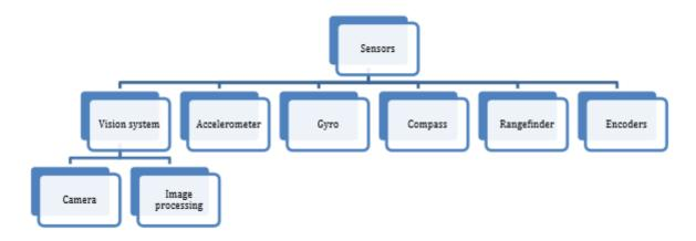
On the cRIO, the FPGA implements all the high speed measurements through dedicated hardware ensuring accurate measurements no matter how many sensors and motors are connected to the robot. This is an improvement over previous systems, which required complex real time software routines. The library natively supports sensors in the categories shown below:
