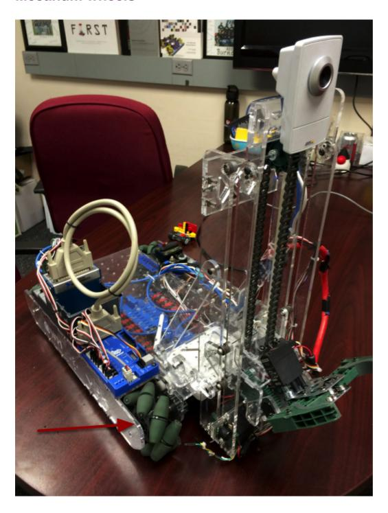
The wheels shown in this robot have rollers that cause the forces from driving to be applied at a 45 degree angle rather than straight forward as in the case of a conventional drive. You might guess that varying the speed of the wheels results in travel in any direction. You can look up how mecanum wheels work on various web sites on the internet.
