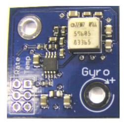
The Gyro object should be created in the constructor of the **RobotBase** derived object. When the Gyro object is used, it will go through a calibration period to measure the offset of the rate output while the robot is at rest to minimize drift. This requires that the robot be stationary and the gyro is unusable until the calibration is complete.
