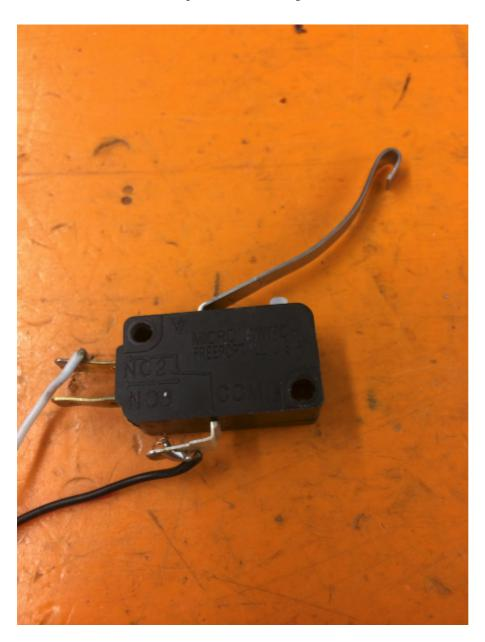
Limit switches can have "normally opened" or "normally closed" outputs. The usual way of wiring the switch is between a digital input signal connection and ground. The digital input has pull-up resistors that will make the input be high (1 value) when the switch is open, but when the switch closes the value goes to 0 since the input is now connected to ground. The switch shown here has both normally open and normally closed outputs.
