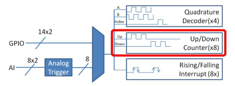
There are 8 Up/Down Counter units contained in the FPGA which can each operate in a number of modes based on the type of input signal:
