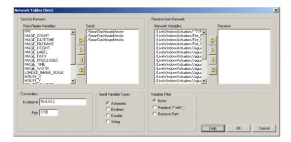
RoboRealm is a program that does client-side (PC) vision processing. RoboRealm can connect to a camera on a robot and do real-time tracking of field targets and sending the results back to the robot. In the past this required writing custom networking code for the PC to robot communications. RoboRealm now has a built-in NetworkTables client and this allows the RoboRealm program to send values directly back to the robot via some shared variables.
