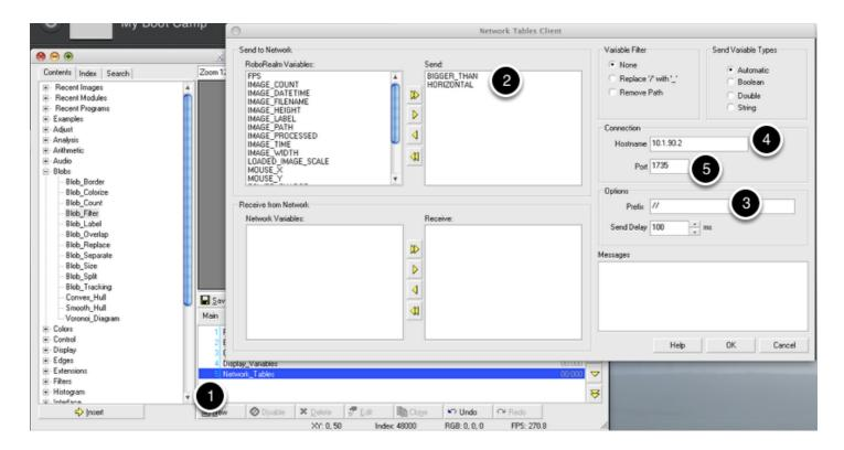
Variables that are created in RoboRealm can be sent back to the robot using NetworkTables. To do that add a "Network\_Tables" step (1) to your RoboRealm program and add the variables you defined to be sent to the robot (2). Set the "Prefix" to "//" (3) and the "Hostname" to the value of your robot network address (4) and the port to 1735 (5).
