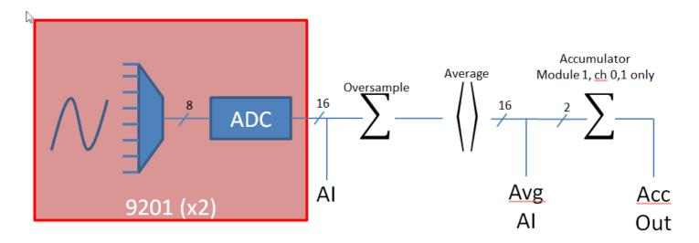
When the system averages a number of samples, the division results in a fractional part of the answer that is lost in producing the integer valued result. Oversampling is a technique where extra samples are summed, but not divided down to produce the average. Suppose the system were oversampling by 16 times – that would mean that the values returned were actually 16 times the average. Using the oversampled value gives additional precision in the returned value.
