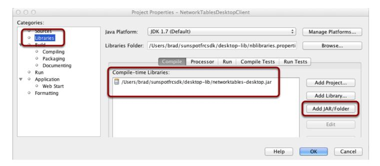
To write a program that runs on your PC that uses NetworkTables the Java project must reference the JAR file from the NetBeans installation shown above. The project has to reference the networktables-desktop.jar file. This is an example of doing it with NetBeans but any IDE will have a way of adding .JAR files to a project. In this example the .jar file was added to the project properties.
